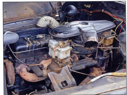
Compound carburetors were optional on 1942 Specials. This one has it.
